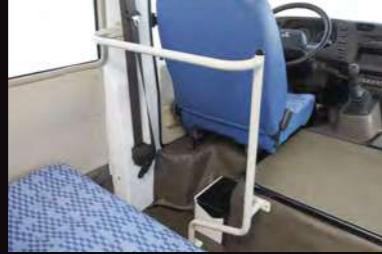
Partition on the backside of the driver seat
