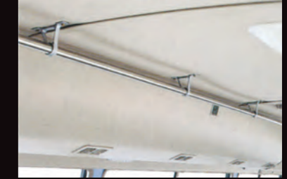
Ceiling grab rail
